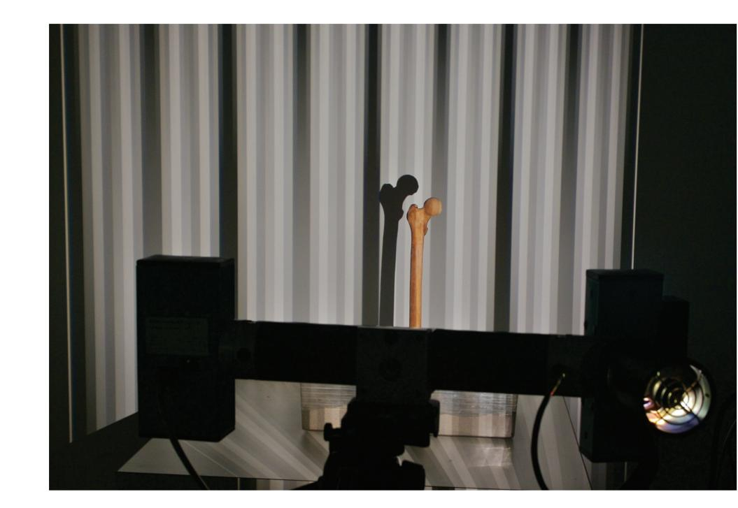
Figure 1. Facing the scanner from behind while projecting the Gray-code onto the femoral surface.
